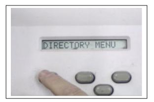
Turn machine on and Put boot disk into drive then hit enter – you will see booting disc Once that is finished, take out boot disk and stick in a disk with a EXP design on it (Melco Expanded) The screen will end up on Directory – you need to hit enter to read the contents of the disk –
